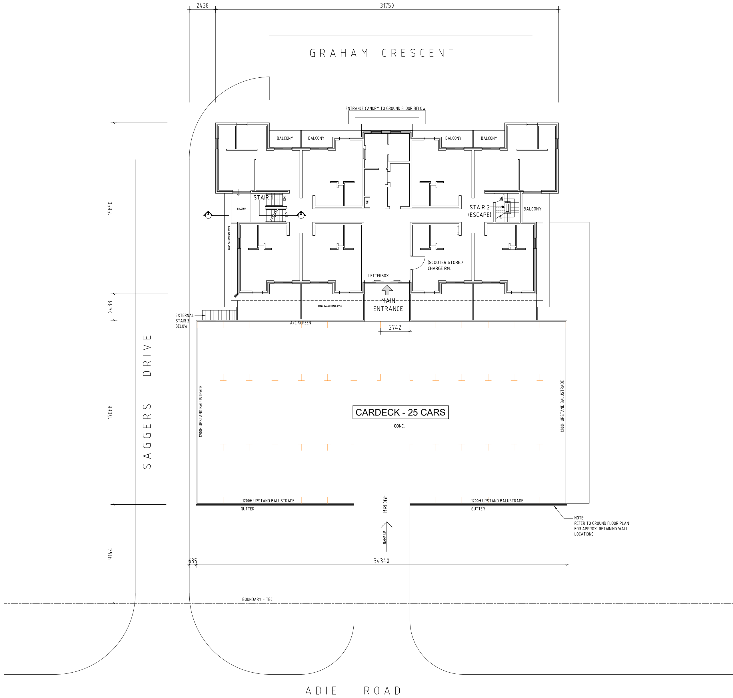
Site Plan at First Floor Level scale 1:200
